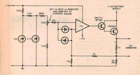
Most digital voltmeters and digital multimeters do not incorporate a milliohms range in their design. This circuit attachment extends the range of any DVM or DMM to measure low resistance, such as RF chokes of transmitters, motor and transformer windings
